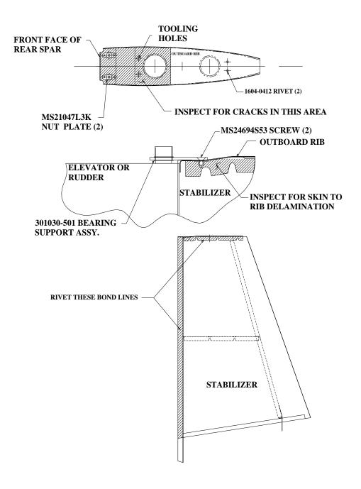
FIGURE 4 STABILIZER OUTBOARD RIB INSPECTION AND RIVET AREA AA1 SERIES & AA5
